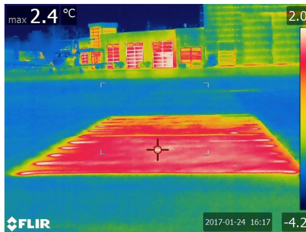
169 170 Figure 2. Thermal image of the ECON HPS slabs at DSM in an experimental test under an 171 average ambient temperature of 0 °C and average wind speed of 4.1 m/s measured at a height 172 of 10 m
