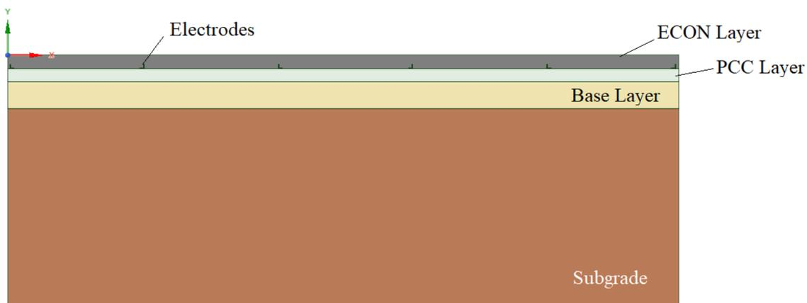
**Fig. 3** Schematic illustration of the pavement layers for electrically conductive heated pavement system test slabs built at Des Moines International Airport
