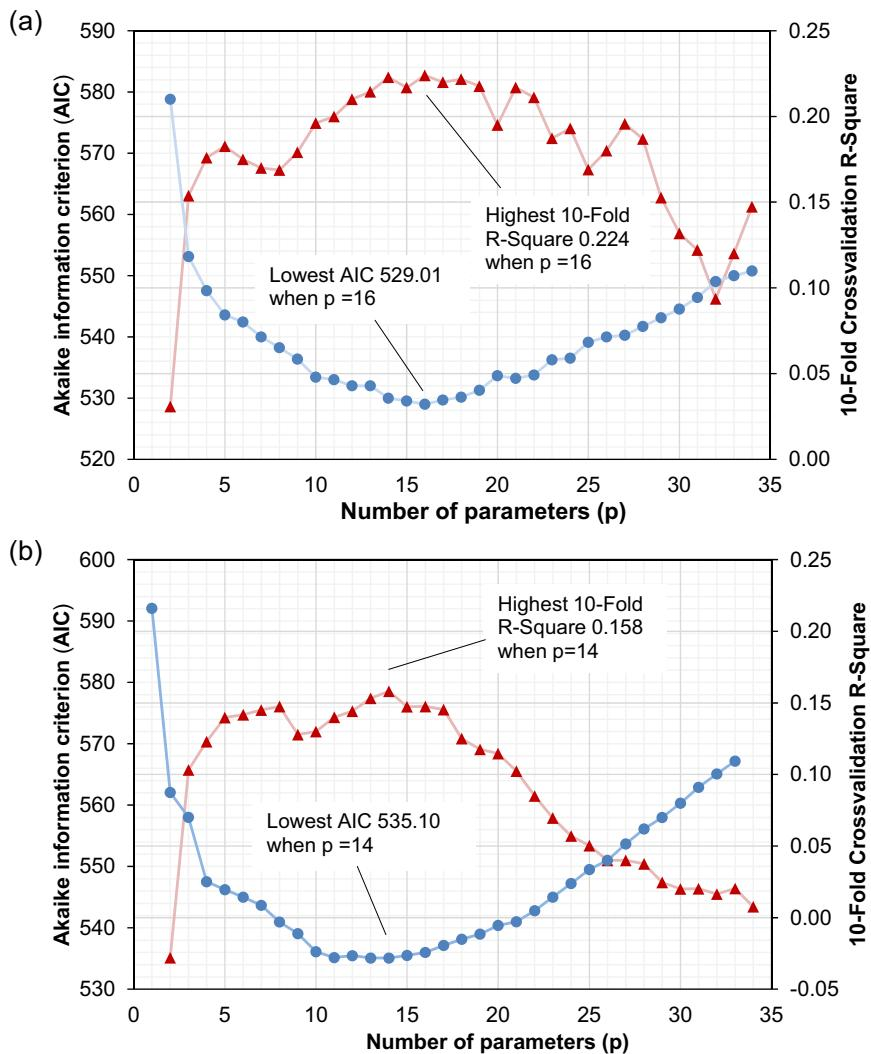
**Fig. 5.** Results of Stepwise Regression Model fits where building technology is presented in (a) Computed Energy Consumption and (b) HERS index.**Table 6**
