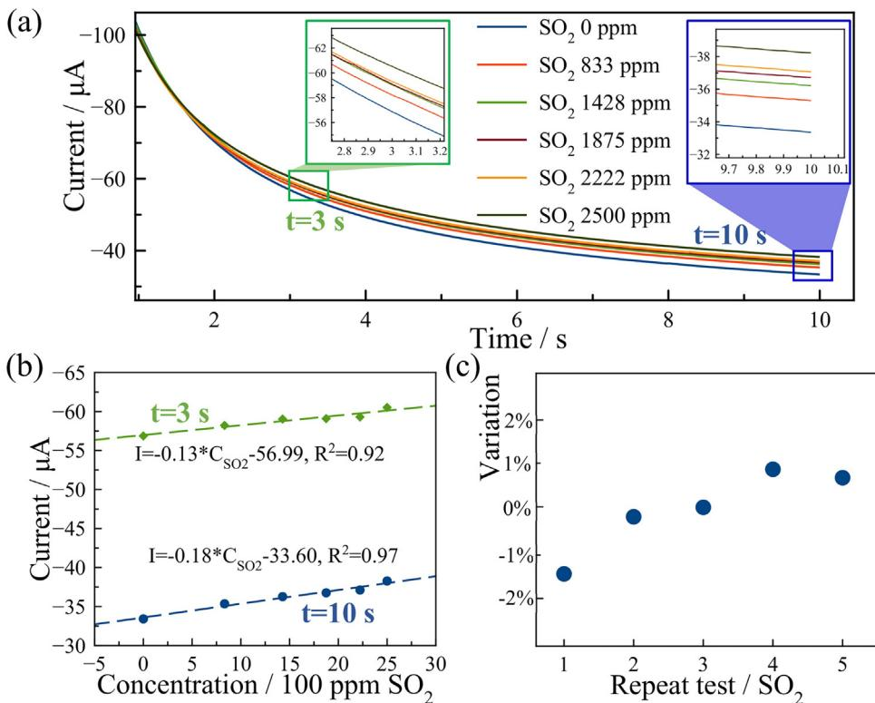
**Fig. 8.** Sulfur dioxide measurement: (a) The current response of the MPRE sensor in  $\text{SO}_2$  measurement; (b) The calibration of the sensor using currents at 3 s (green) and 10 s (blue); (c) The relative variation of five repeat tests using currents at 10 s in 2222 ppm  $\text{SO}_2$ . (For interpretation of the references to colour in this figure legend, the reader is referred to the web version of this article.)
