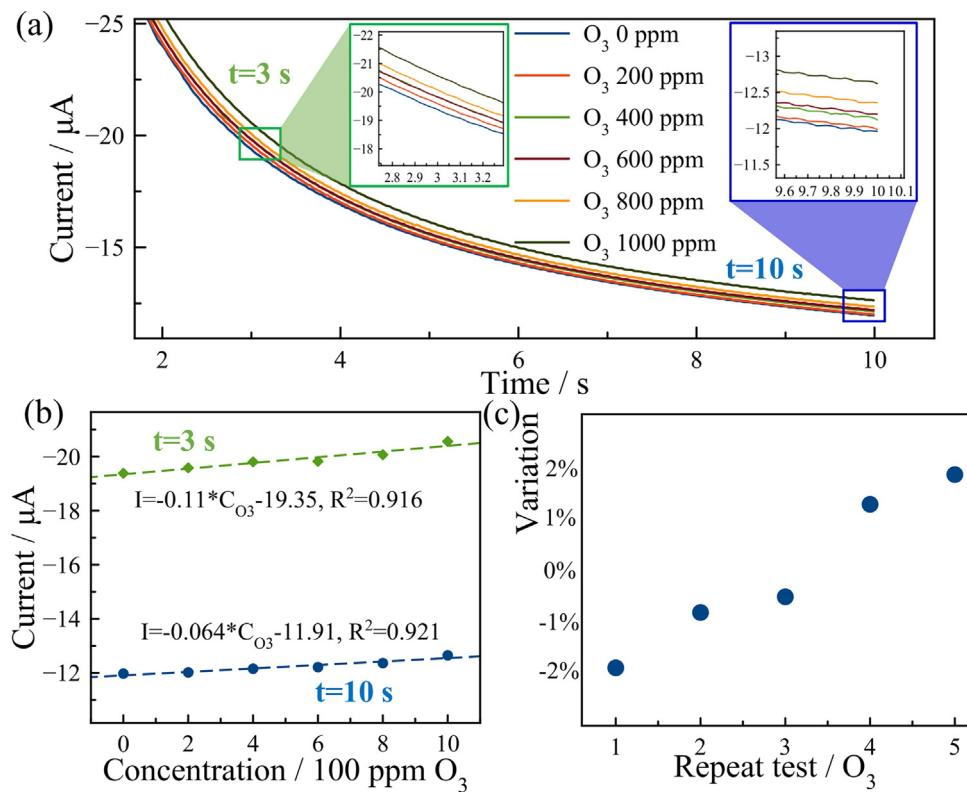
**Fig. 9.** Ozone measurement: (a) The current response of the MPRE sensor in  $\text{O}_3$  measurement. (b) The calibration of the sensor using currents at 5 s (green) and 10 s (blue); (c) The relative variation of five repeat tests in 800 ppm  $\text{O}_3$ . (For interpretation of the references to colour in this figure legend, the reader is referred to the web version of this article.)
