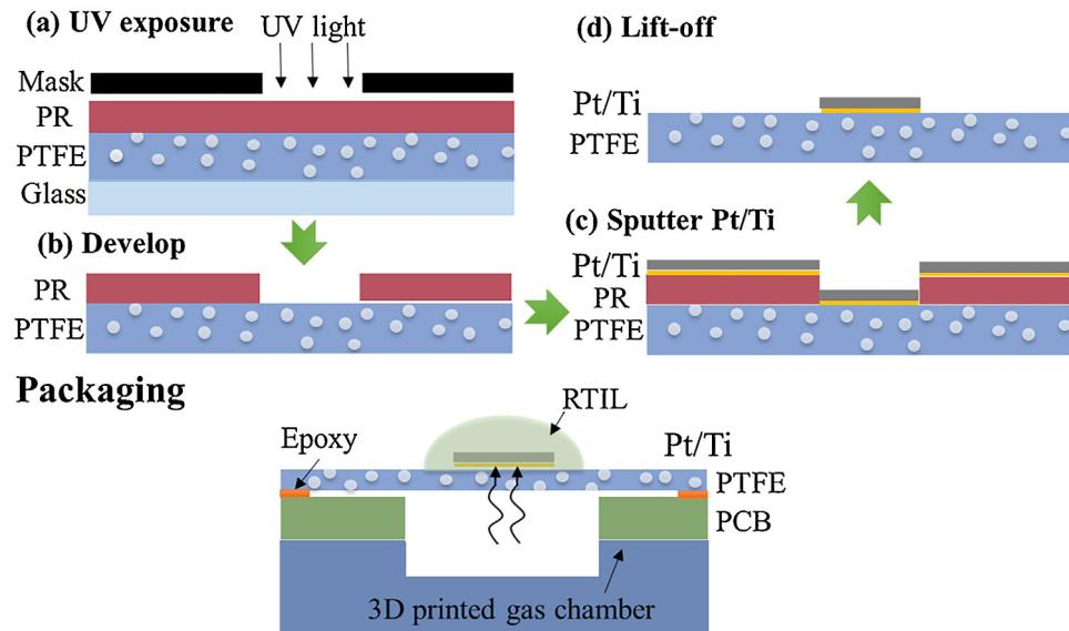
**Fig. 3.** The microfabrication process and packaging of the MPRE sensor: (a) UV exposure; (b) Develop; (c) Sputter Ti/Pt; (d) Lift-off.
