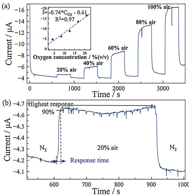
**Fig. 5.** The oxygen response of the MPRE sensor: (a) Current response for chronoamperometry at  $-1.2\text{ V}$ ; (b) Calculation of response time for 20% air change. The inset of (a) shows the calibration plot of current vs. oxygen concentration.
