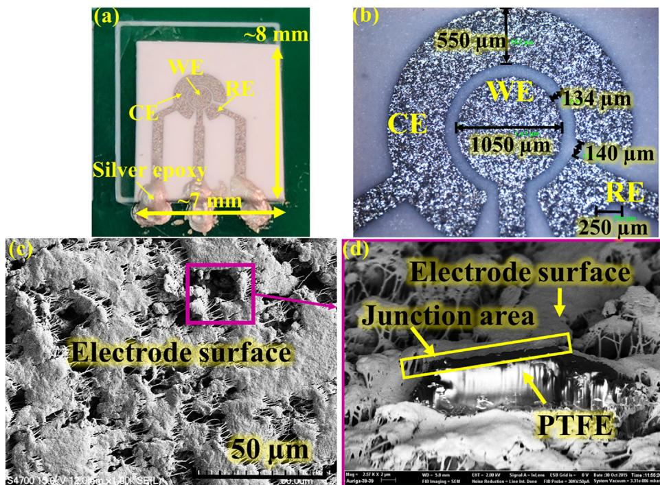
**Fig. 4.** The photo of the MPRE sensor and inspection of electrodes: (a) The photo of two packaged sensor on PCB; (b) The photo of the electrodes by optical microscope; (c) The SEM image of platinum electrode topography and (d) a side view of a rough spot on the electrode using FIB.
