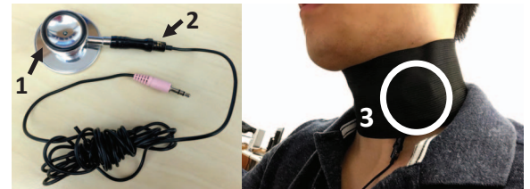
Fig. 8: The hardware for audio-based sensing. (1) A chestpiece of a clinical Elite 4000 stethoscope. (2) A unidirectional condenser microphone. (3) The chestpiece attached to skin using an elastic band.
